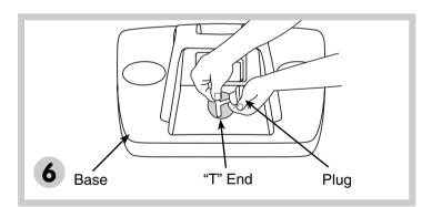
Bend the "T" end of the plug and insert it into the hole in the base.
